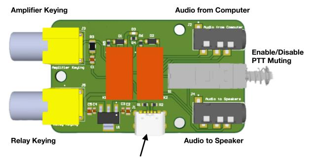
**USB-C Connector for Power 5VDC**
